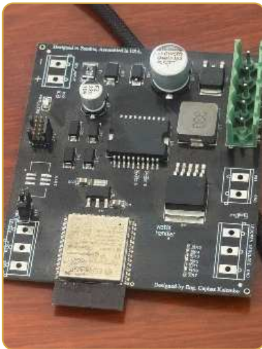
Oil-pump controller , designed here by our founder for a Texas client. Printed on the board: "Designed in Zambia".
