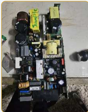
A rectifier module opened on the bench.
